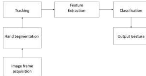
Figure.1 Block diagram of the proposed methodology
